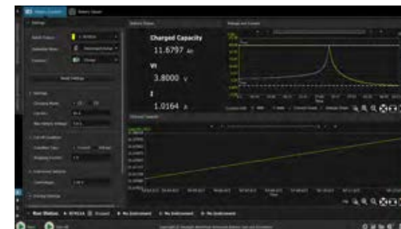
Figure 5. Visually tracking battery charging using BV9210B / 11B software
